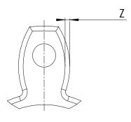
If the measured value (Z value) is higher than that indicated in the Z VALUE FOR CHECKING SPIDER WEAR, it is recommended to replace the spider with an equivalent one.
