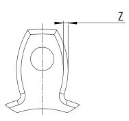
If the measured value (Z value) is higher than that indicated in the <u>Z VALUE FOR CHECKING SPIDER WEAR</u>, it is recommended to replace the spider with an equivalent one.
