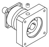
G. Re-install the access hole plug into the motor adapter plate. Assembly is complete.
