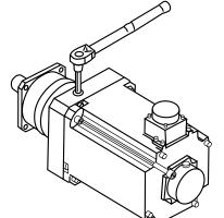
F. Tighten the gearbox input shaft clamb bolt to the proper torque using a torque wrench (see Table B).
