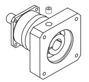
A. Remove the access hole plug, allowing access to the motor shaft clamp.
