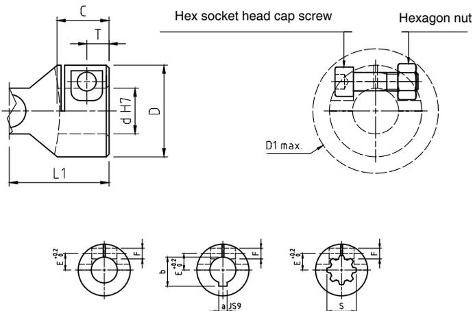
Type 2: clamping hub + lock nut seat
