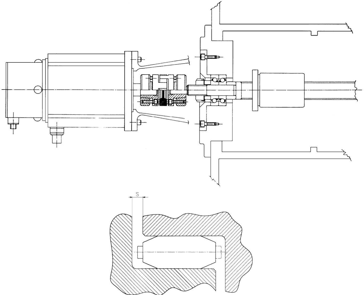
With the A and AP versions, mounting the hubs can be facilitated by lubricating the shaft contact surfaces with an oil, but **do not use a molybdenum bisulphide based oils**. When mounting the TRASCO® ES coupling an axial thrust is generated which disappears when the mounting has been completed to avoid putting axial loads on the bearings. Lubrication of the elastic element will reduce the amount of axial force required during installation.
