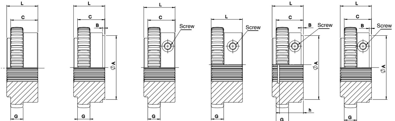
**Fig.1** Splined bore hub
