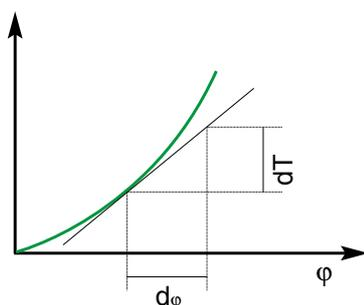
Dynamic torsional rigidity  $C_{Tdin}$  is the first derivate of the nominal torque of half coupling in respect to the torsion angle.
