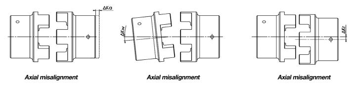
Figure 2-9 - TRASCO®: misalignments
