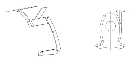
If the measured value (Z value) is higher than that indicated in the Z VALUE FOR CHECKING SPIDER WEAR, it is recommended to replace the spider with an equivalent one.
