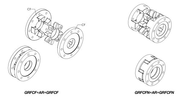
Figure 4-5 - Flange-flange version (CF/CFN)
