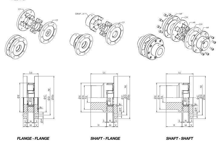
Figure 2-4 - GRF TRASCO® Hubs
